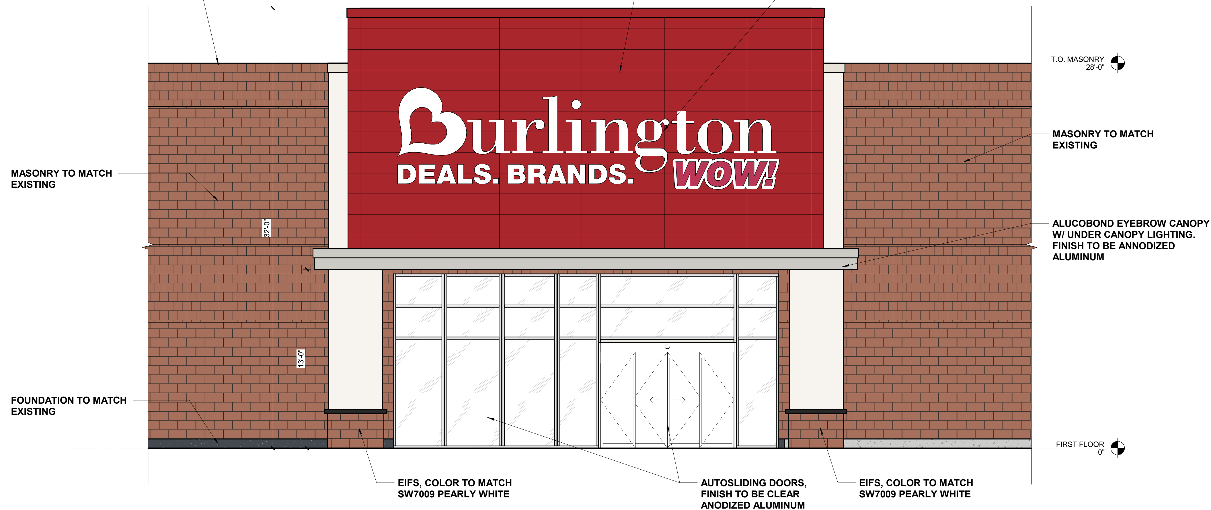
ENLARGED EXTERIOR ELEVATION - FRONT FACADE 1/4" = 1'-0"
