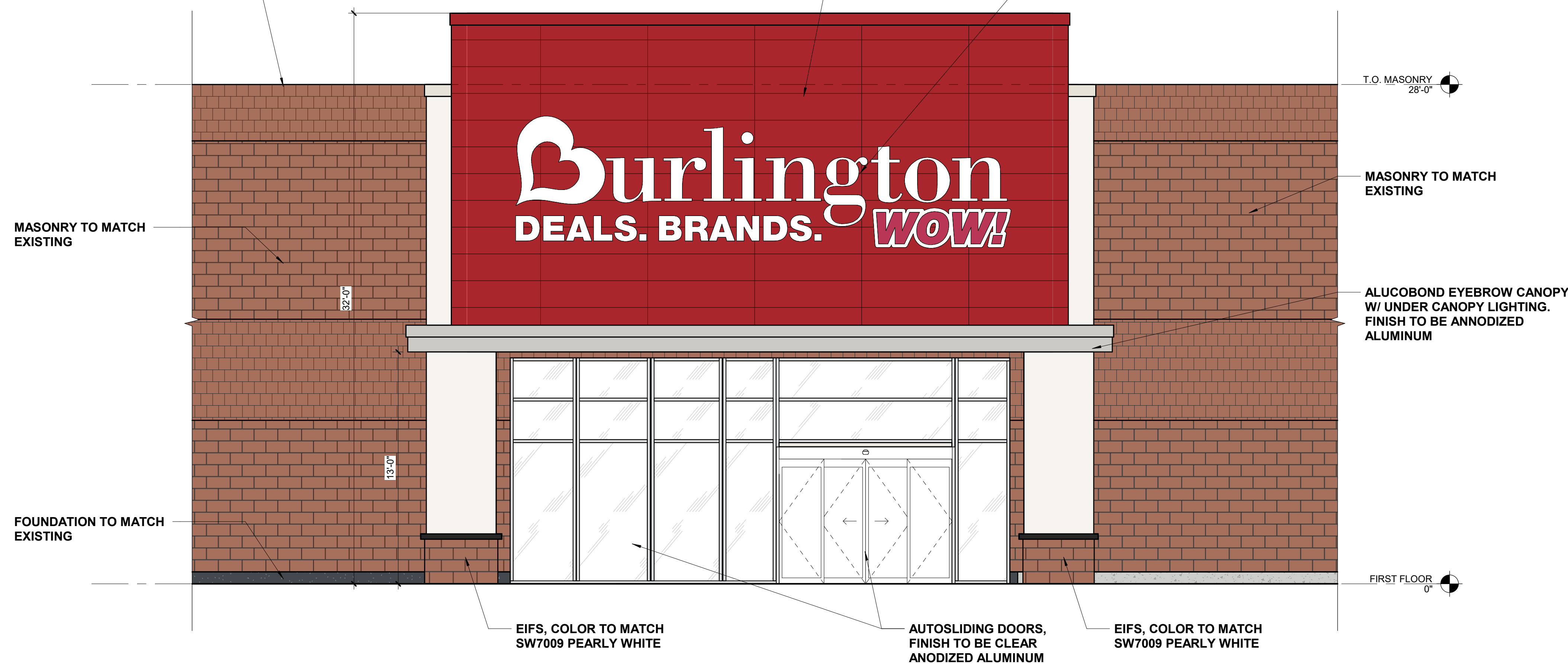
ENLARGED EXTERIOR ELEVATION - FRONT FACADE 1/4" = 1'-0"
