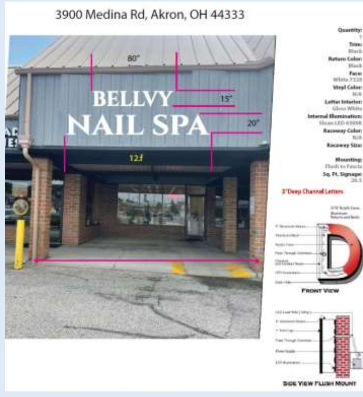
The sign is comprised of channel letters with white acrylic faces placed on aluminum returns flush mounted to the wall.
